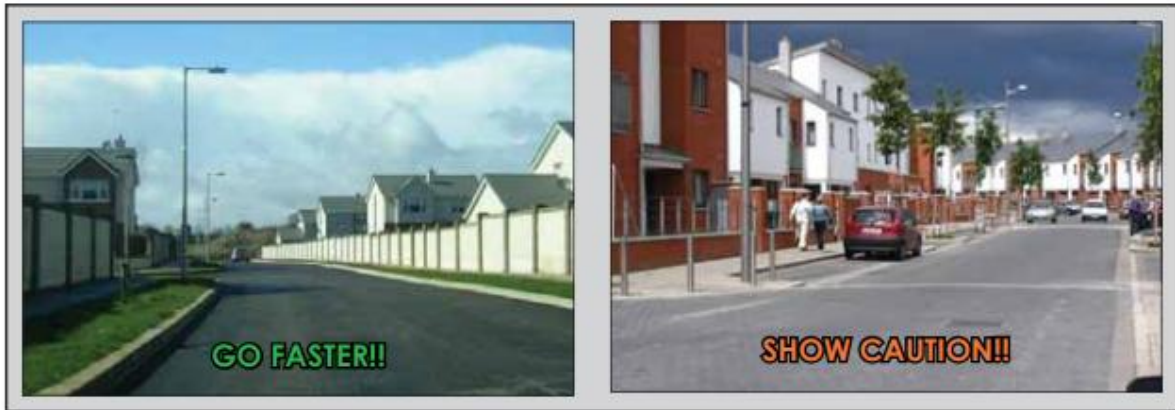
Figure 5: The elimination of access and frontage along roads was introduced to reduce risk, but it serves to encourage speeding (DMURS, 2013)
